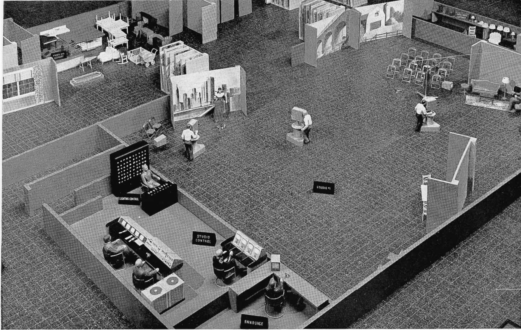
FIG. 52. View of large Studio #1, companion control room and the nearby "prop and scenery" storage area. Note that, in this setup which uses the TC-5A Program Director's Console, the video monitors have been located away from the control room window. The program director and audio operator are at a second level, with the lighting control operator and his equipment plus the video monitors at a lower level. (Actually these camera controls could be located in a different room.)
