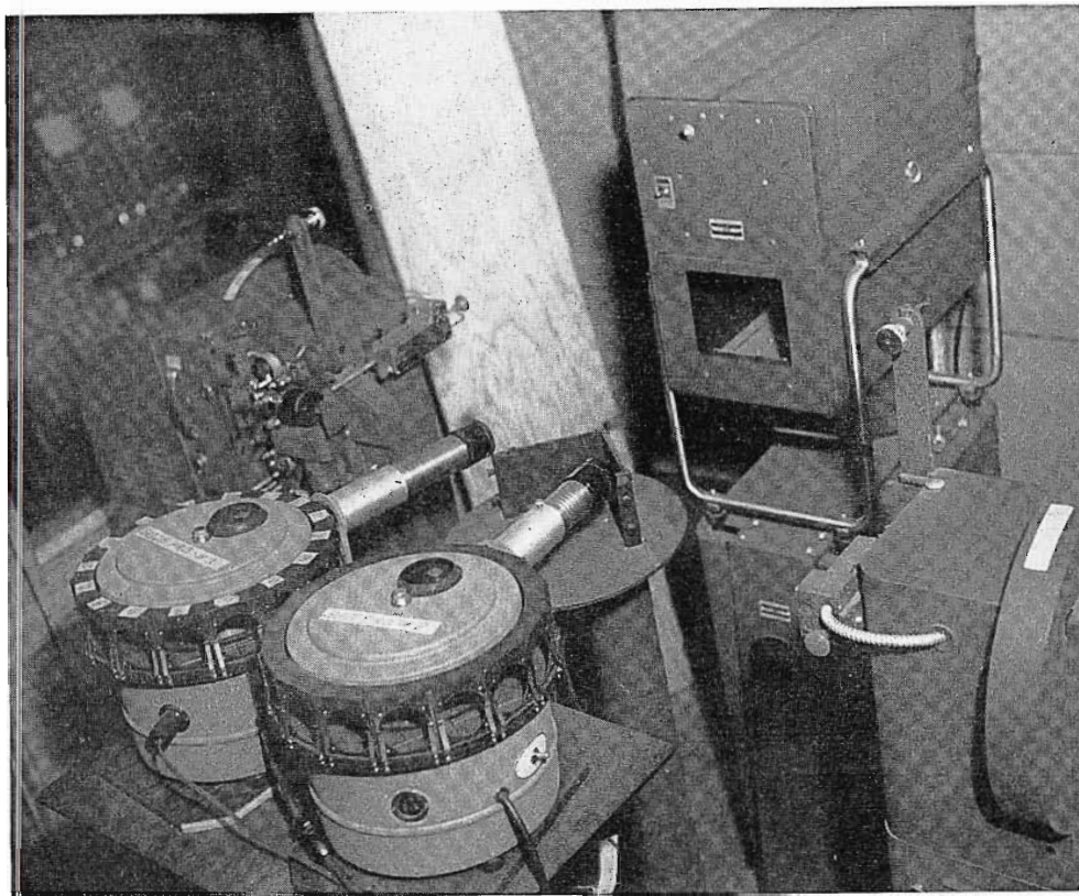
FIG. 5. Film facilities utilize two RCA TP-16D Projectors, TK-20C Film Camera and two automatic slide projectors.
