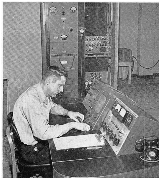
FIG. 8. WSBT-TV Engineer, Howard Paulsen, is shown seated at the RCA TTC-1B transmitter control console. Sufficient blank space is left in the rack to receive a demodulator and sideband response analyzer.
